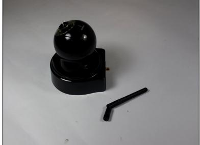
Unscrew the antenna in a counter-clockwise rotation.
