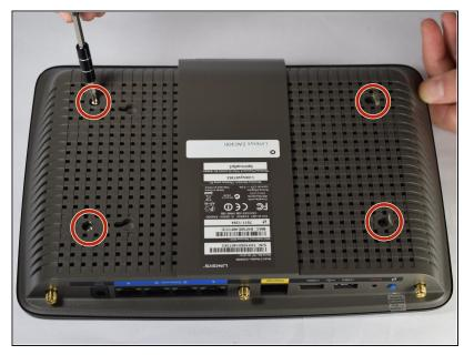
Remove the 0.4cm head screws from each slot with the #1 Phillips head Screwdriver.
