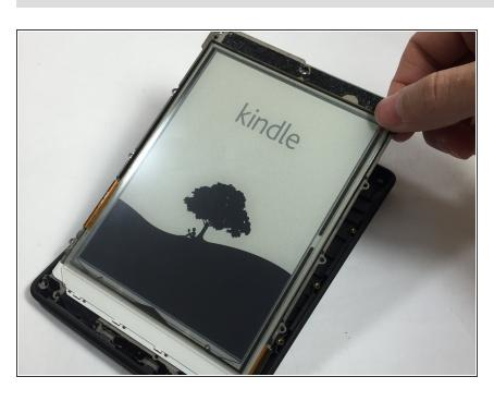
Carefully lift and remove the midframe.
