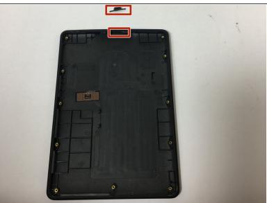
Remove the power button carefully using a blue plastic opening tool, and replace with a functional unit.
