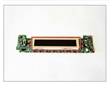
Please refer to the <u>iFixit soldering</u> guide for help removing the LCD screen.
