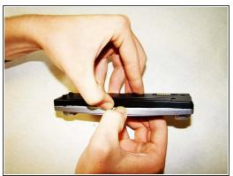
Use two fingers to create a small gap on the top of the faceplate, as indicated in the picture.
