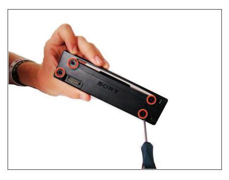
Unscrew the four (length - 11.11mm) phillips-head screws on the front screen.
