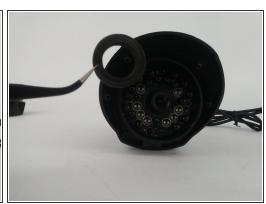
Remove the LED foam ring with tweezers.
