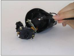
• Use tweezers to disconnect the microphone wires from the internal components of camera.
