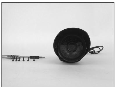
Remove the six 10mm Torx T10 screws on camera face.
