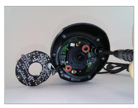
Remove the two 5mm Phillips #1 screws.
