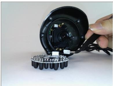
Use tweezers to unclip the cables to the LED board
