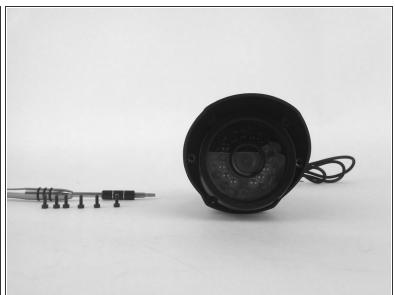
Remove the six 10mm Torx T10 screws on the camera face.
