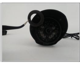
Remove the LED foam ring with tweezers.
