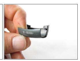
Use a plastic opening tool to gently pry the bottom cover loose.
