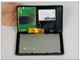
Open the device carefully being weary of the orange band that is going from the screen to the mother board.
