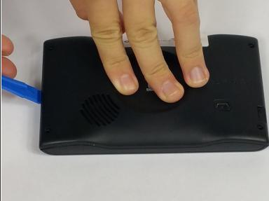
Use the plastic opening tool on all four sides of the device to open the Garmin Nuvi LMT2455 Back Panel.
