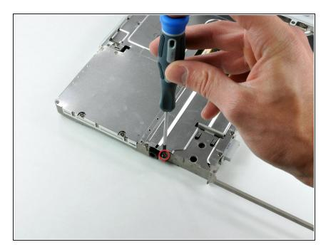
Remove the single Phillips screw securing the sleep light to the metal framework.
