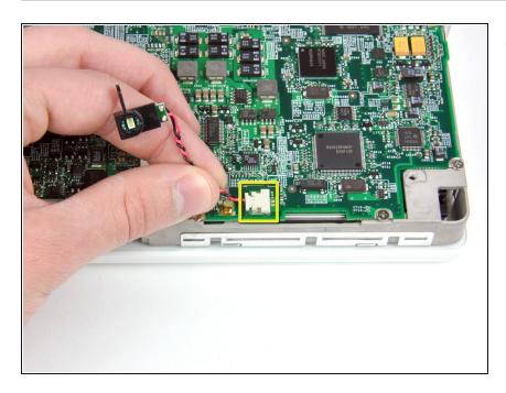
Turn the computer over and disconnect the sleep light from the logic board.
