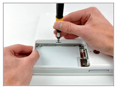
There is a slot on the wall of the battery compartment that locks the lower case in place. Use a small flathead screwdriver to pry out the slot's lower rim and pull up on the lower case to free the slot from the tabs holding it.
