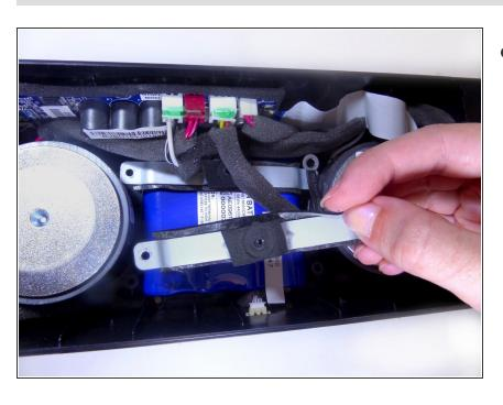
Remove the two brackets that hold down the battery using your hands.
