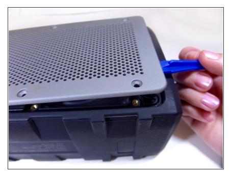
Lift the back panel off of the device with a plastic opening tool.
