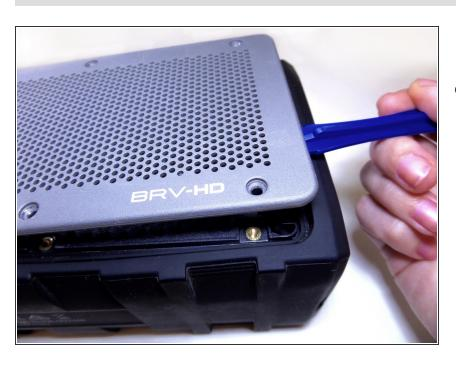
Lift the front panel off of the speaker using a plastic opening tool.
