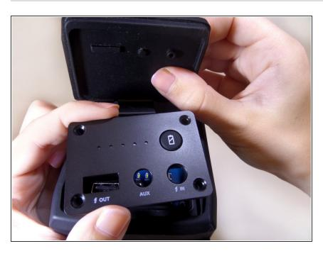
Remove the outer rubber flap and the plastic side port panel.
