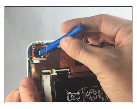
Remove the ribbon cord from its slot using a plastic opening tool.
