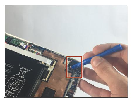
Lift the retaining flap fastening the ribbon cord to the motherboard using a plastic opening tool.
