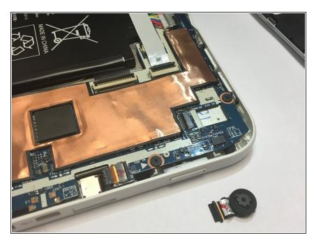
Remove the rear-facing camera from its slot and pose for a camera shot.
