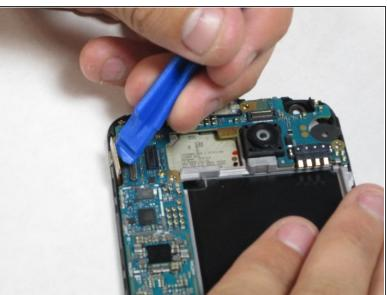
• Insert the plastic opening tool between the screen-ribbon-connector and the motherboard, then pull up. It should pop out easily.
