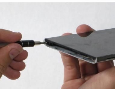
Remove the two 5.5mm Phillips #00 screws from the base of the phone.
