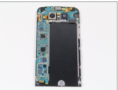
Peel the screen away from the body. The two parts should be completely separated.
