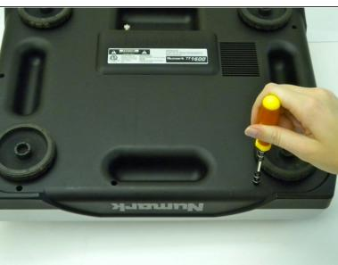
Flip over the turntable and remove the nine screws on the outer edges.
