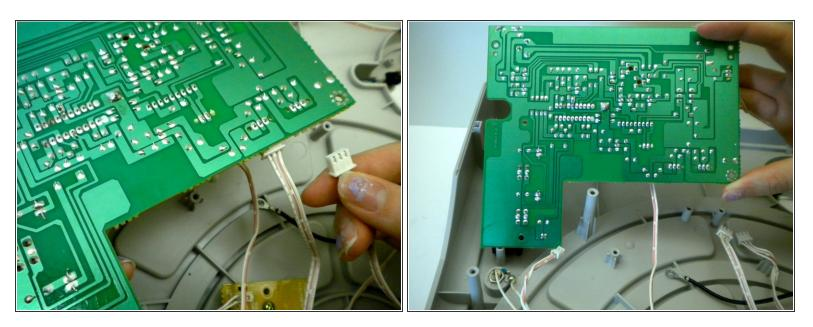
Gently pull out the wires plugged into the circuit board.
