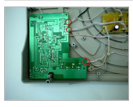
Locate the wires that are plugged into the side of the circuit board.
