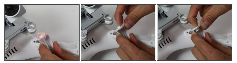
Remove the rubber spacer in the landing gear by pushing the spacer out of the slot with your finger.
