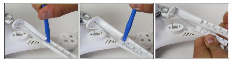
• Using a plastic opening tool, carefully separate the two pieces of plastic of the landing gear.
