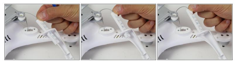
• Feed the wire and attached plastic through the hole in the landing gear.
