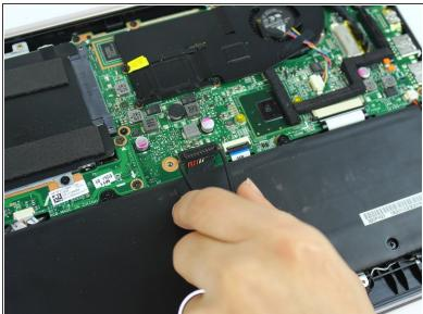
Remove the ribbon cable with a pair of tweezers.
