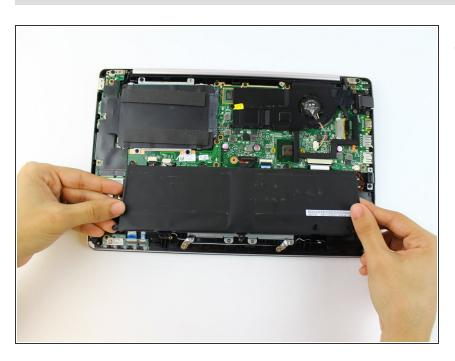
Lift and remove the battery.
