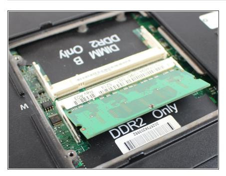
Carefully pull the ram modules out of it's slot, away from the motherboard.
