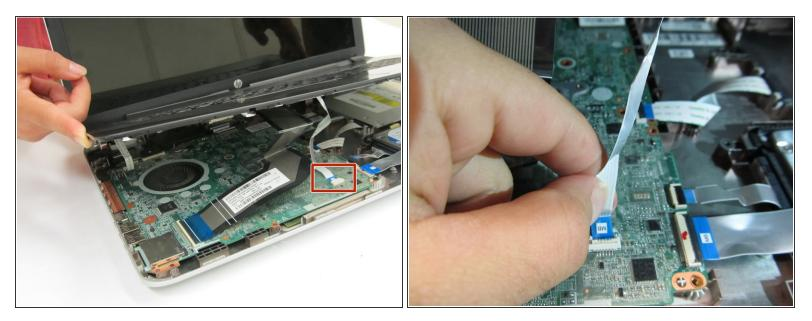
• Remove the ribbon connecting the mousepad to the motherboard.
