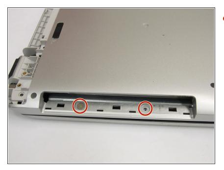
Remove two 2.4 mm broadhead screws from the CD Drive bay with a Phillips #0 screwdriver.
