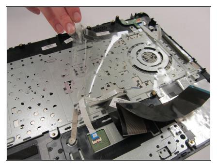
• Turn the front panel over and partially remove the clear plastic covering the keyboard casing.
