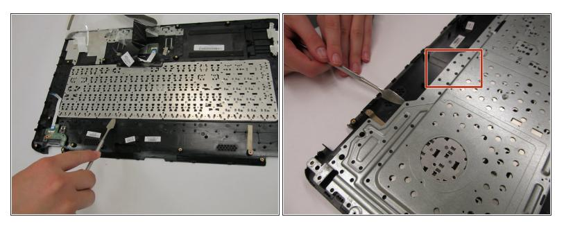
A Plastic debris may scatter while lifting the metal housing. These pieces are indicated in red.
