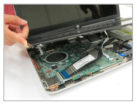
• Partially lift the top cover from the enclosure.
