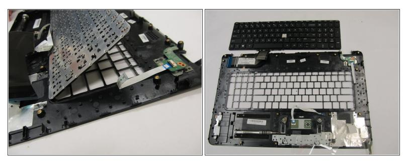
• Lift the metal housing from the front panel to separate the keyboard from the top panel.
