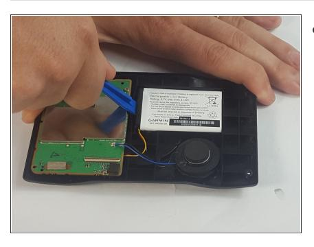
Using the plastic opening tool, pry the battery from the base of the device.
