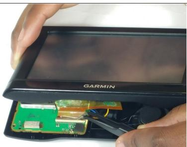
Remove the orange band from the motherboard to access screws.
