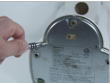
Remove the three 16 mm tri-point screws from the base plate.
