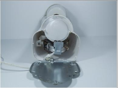
Remove the base plate by pressing the plastic body away from the metal plate with your thumbs.
