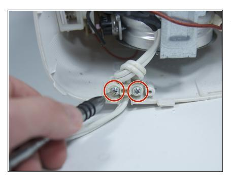
Remove the two 8mm Phillips screws from the plastic body.
