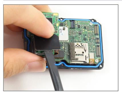
Use the flat end of the spudger to pry the black cover plate straight up from its socket on the motherboard.
