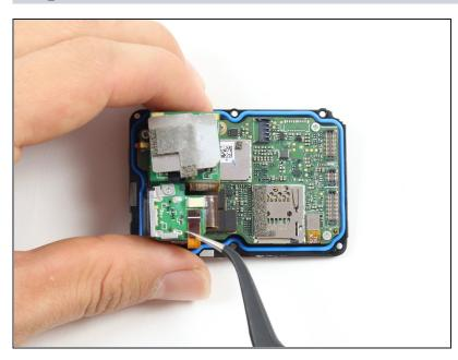
Use the <u>tweezers</u> to pull the ribbon cable connector out of its white socket on the charging assembly board.
