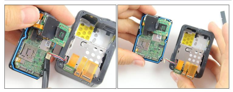
• Use the flat end of the spudger to pry the battery housing power cable straight up from its socket on the motherboard.
