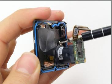
• Remove the 2mm #000 Phillips screws using a #000 Phillips head screwdriver or tool bit.
