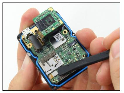
Use the flat end of the spudger to pry the LCD screen ribbon cable connector straight up from its socket on the motherboard.
