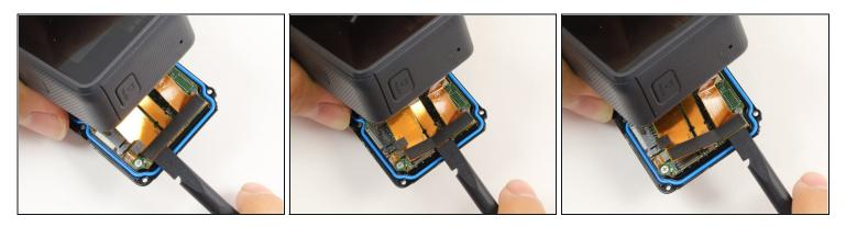
• Use the flat end of a spudger to pry the three ribbon cables connected to the side of the motherboard.
