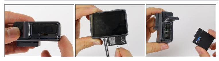
• Grab the plastic flap on the battery and pull the battery out.
