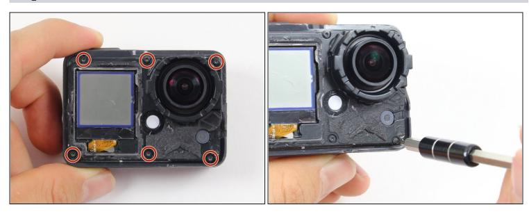
Remove the six T3 Torx screws.
