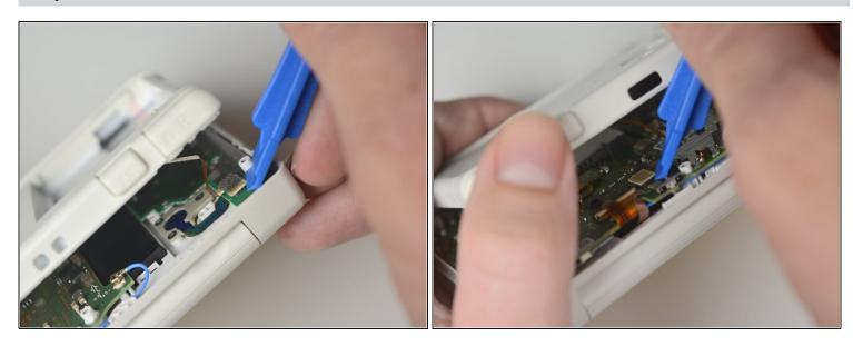
Lift the top edge of the lower case slightly off on the 3DS.
