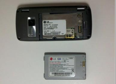
Simultaneously lift the battery out of the phone.
