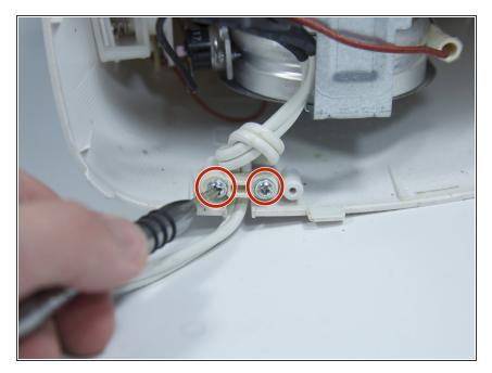
Remove the two 8 mm Phillips screws from the plastic body.
