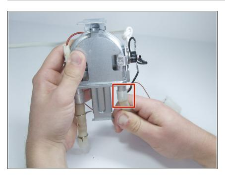
Remove the two rubber water tubes from the heating element by firmly pulling each at a 90 degree angle from the socket.
