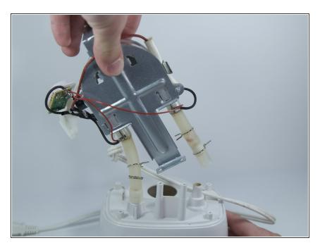
Bend the heating element back and forth to wiggle the water tubes loose from the plastic.
