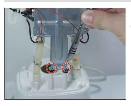
Remove the two 8 mm Phillips screws from the metal backing.
