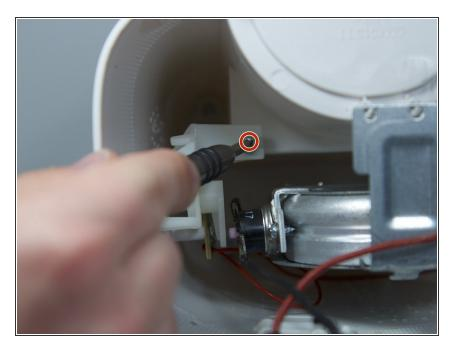
Remove the 8mm Phillips screw that attaches the power button to the inside of the coffee maker.
