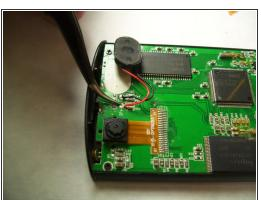
• Use the <u>soldering guide</u> to desolder the speaker contacts.
