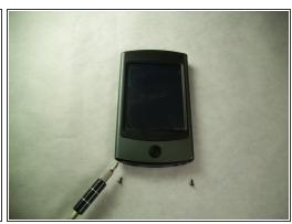
Using the screwdriver with the J00 bit, remove the two 4.8 mm Phillips screws.
