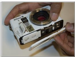
Using the Phillips PH00 screwdriver, remove the six 4.0mm screws marked in red. Then remove the panel cover by lightly pulling it off.
