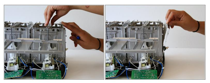
• Pull the metal sheet away from the toaster to expose the heating board.
