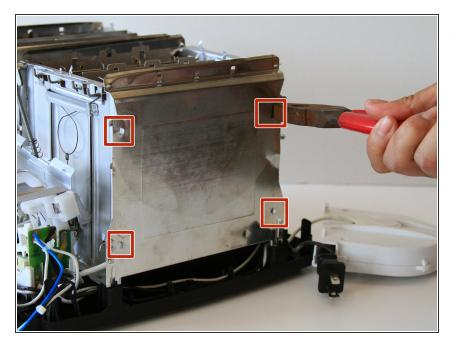
• Position the 4 side tabs to fit thought the slots.
