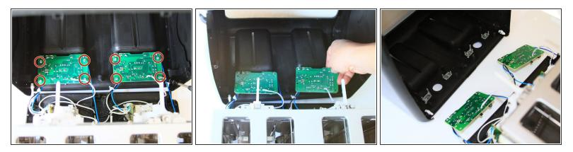
• Use a J1 screw bit to unscrew eight 8mm screws from the motherboard.
