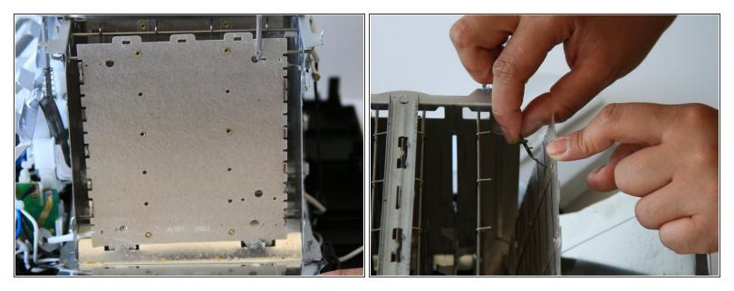
• Position the 4 metals tabs on the heating board. Found at the top right and bottom left.
