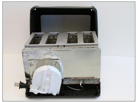
Once the outer shell is removed, rotate toaster so the back is facing you.
