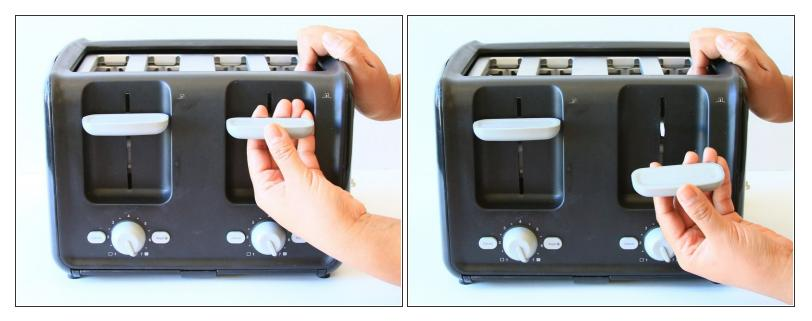
• Forcefully pull the slot lever away from the toaster by keeping parallel to the table.
