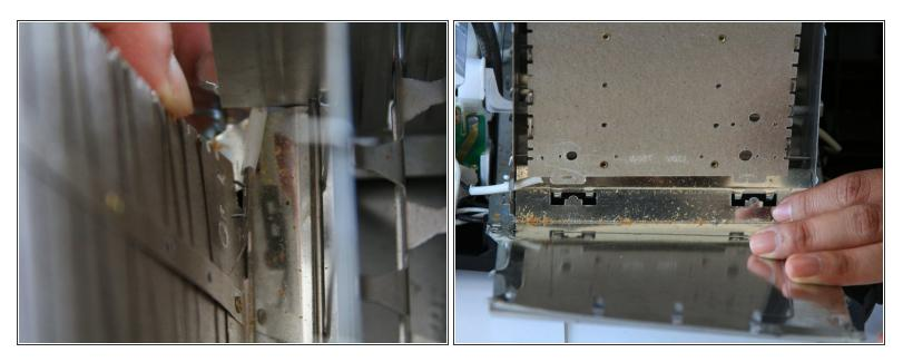
• At the bottom of the heating board, there are 2 tabs holding it to the rest of the toaster, pull those 2 tabs upwards to release heating board from the toaster.
