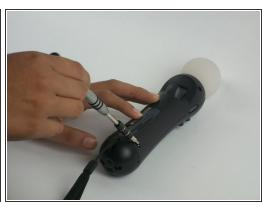
Using a Phillips #0 screwdriver, remove the four 10mm screws located on the back of the device.
