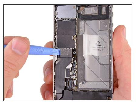
Use the edge of a plastic opening tool to pry the dock cable up from its socket on the logic board.
