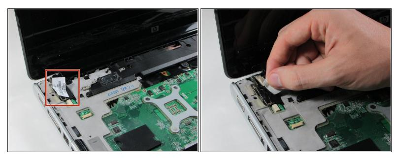
• Disconnect the display cable by lifting the Mylar tab up towards the screen.
