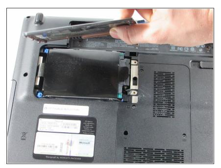
After removing the two screws securing the Hard Drive to the bottom case, remove the panel to reveal the hard drive.
