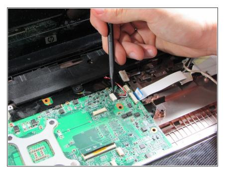
Now disconnect the audio cable (red and white) also using the flat plastic spudger. Gently pry the black piece of the connector away from the white connecting dock it sits in.
