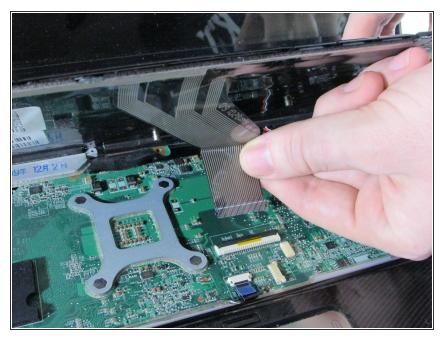
• Remove the film from system board to then safely remove the keyboard.
