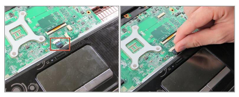
Disconnect the touch pad ribbon cable from the system board by pulling on the blue tab towards you.
