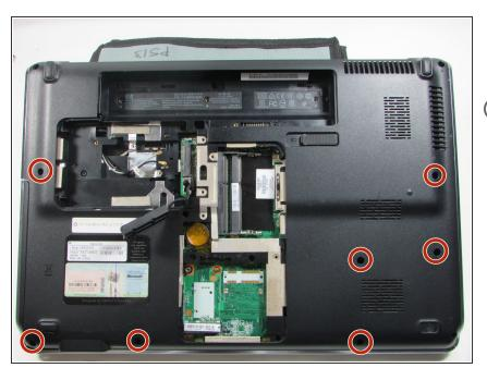
Remove the remaining screws on the bottom of the laptop.
