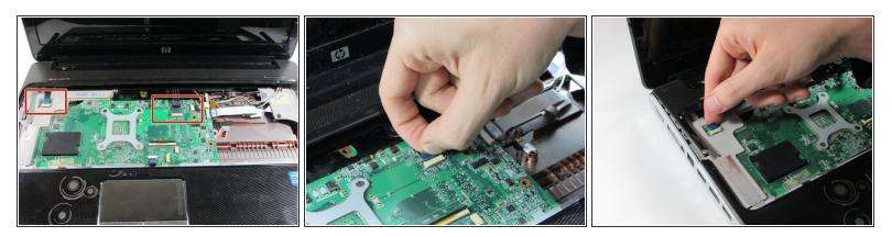
Disconnect the LED board and power button cables from the connector on the system board by pulling the blue Mylar tabs toward the display screen.
