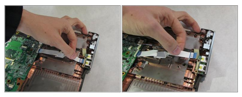
• Locate and disconnect the white and blue USB ribbon cable by grasping the ribbon with index finger and thumb to gently pull away from the USB ports.
