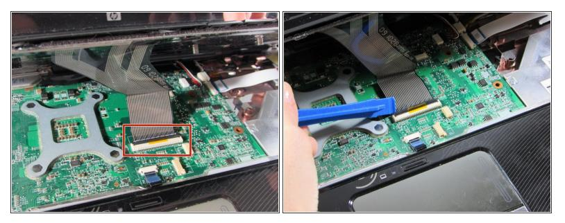
Use plastic spudger to flip up the black strip on the ZIF connector that connects the ribbon cable to the motherboard.
