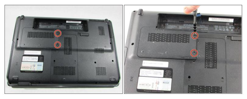
A Shutdown your computer and remove the battery before beginning the replacement.
