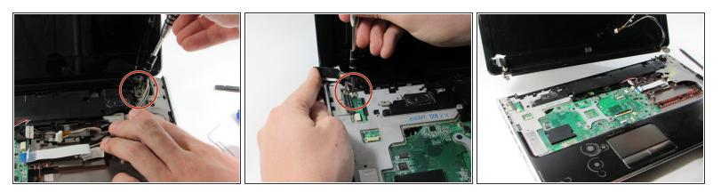
A support the display while removing the screws for this step to avoid damaging the display.
