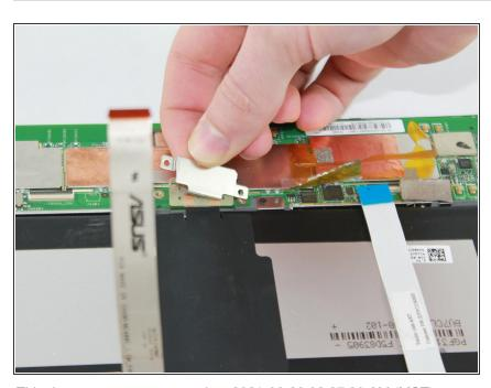
Gently lift the battery pressure plate off of the motherboard.
