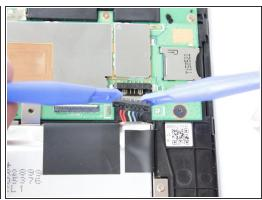
Remove the battery connector by prying it up away from the device using 2 plastic pry tools
