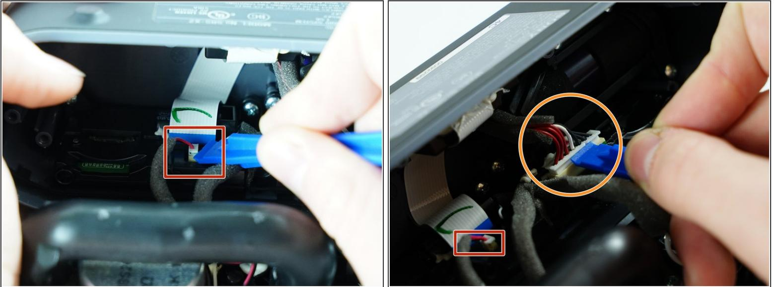
⚠ Be gentle when using the opening tool, wiggle the opening tool on each side of the socket to be sure the plastic does not snap.
