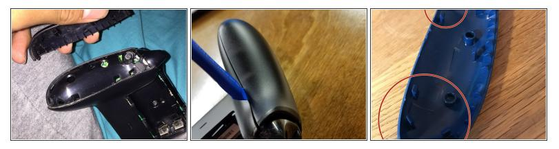
• Remove the side panels exposing the second T8 security screw using a spudger, an IFixit Opening Tool, or your nails, each choice is fun.
