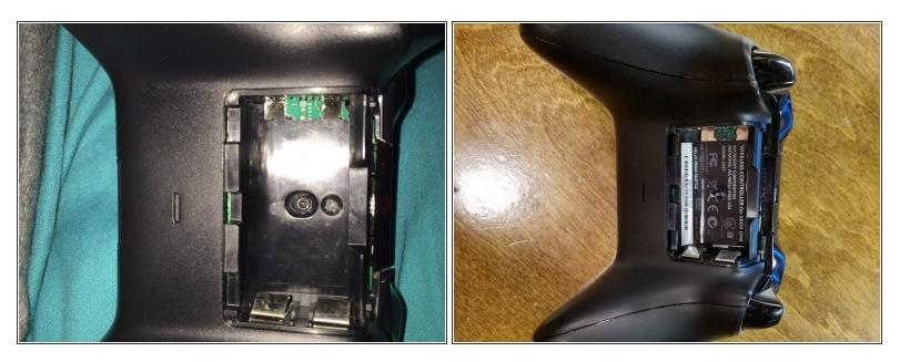
• Start with removing the battery pack and exposing the T8 security screw. The screw should be hidden behind a warranty sticker.
