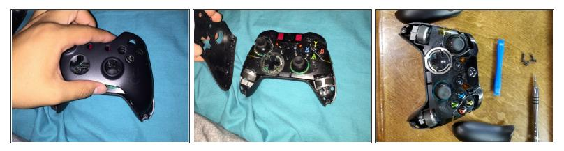
• Once you removed the T8 security screws remove the front face plate.
