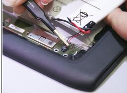
Pull up the battery cables and battery chip with tweezers.
