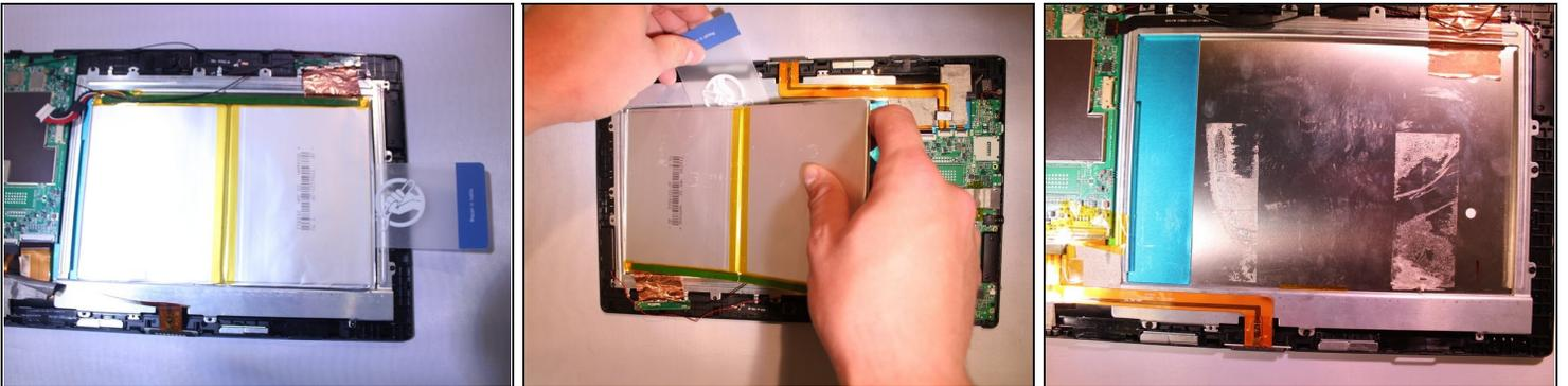
**⚠ Make sure not to bend the battery too excessively as if bent too much, it could rupture a cell within the battery and possibly cause a fire.**
