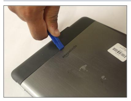
Push an opening tool against the bottom cover edge of the device.
