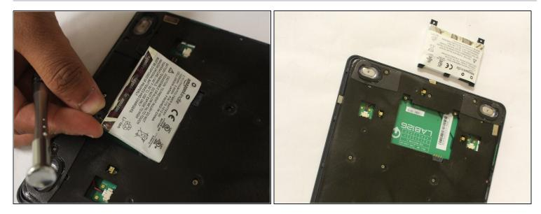
• Remove the battery from the device.
