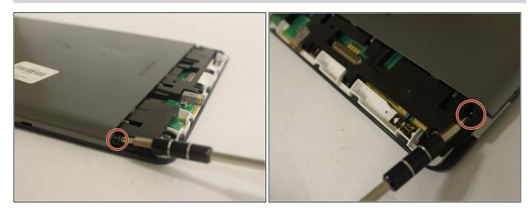
Remove two 40 mm screws (one on each corner) using a Phillips #00 screwdriver.
