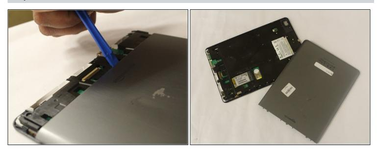
Use the edges of the opening tool, get in between the seams of the front and back panel, and
