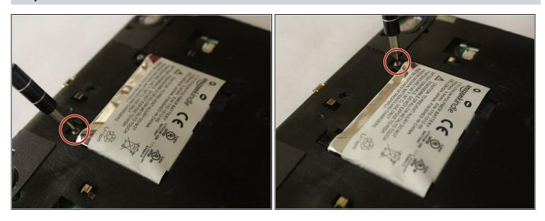
Remove two 30 mm screws securing the battery with a Phillips #00 screwdriver.
