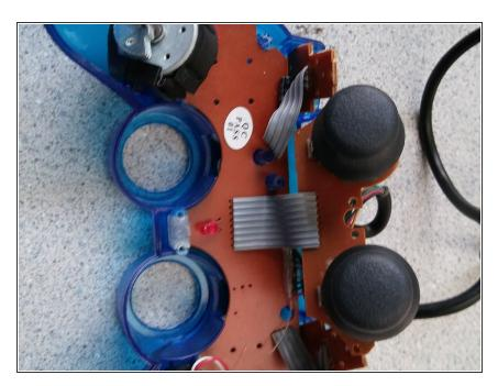
The last step was on the other side of the controllers backside, also the inside and this is where we removed the two sticks and had to put all the screws and pieces back together.
