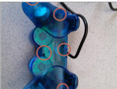
I had to remove all the screws on the back to get the controller open to see the inside or tear it down
