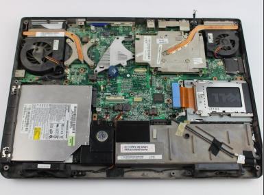
Pull up and away on the track pad to expose the internal components below.
