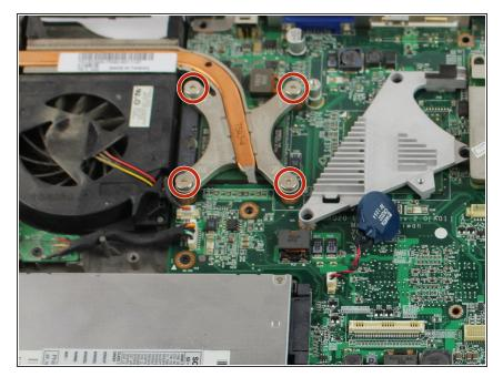
Loosen the four silver Phillips screws in a criss-cross pattern retaining the heatsink to the cpu.
