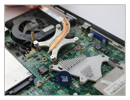
Gently lift up on the heatsink to reveal the CPU below.
