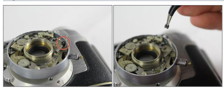
• Remove the stopper by lifting it upwards with the <u>tweezers</u>.
