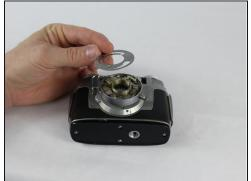
• While the camera is lying on its back, unscrew the front lens assembly and remove the lens and the faceplate. Then lift off the speed setting.
