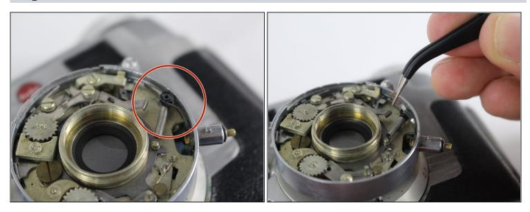
• Remove the lever from the stopper by pushing it back and then upwards.
