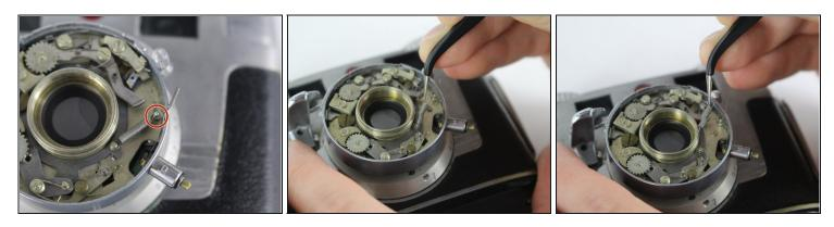
• Using tweezers, unhitch the spring from the base and remove it by lifting upwards.
