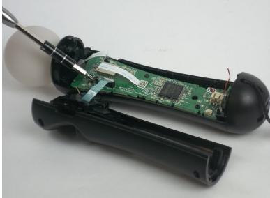
Remove the two 1.2mm Phillips #1 screws.
