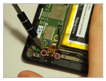
After locating the Aux port at the bottom of the device, remove the (2) 3mm T4 Torx screws.
