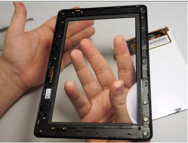
Once the ribbon and screws are removed, pick the part up and tilt it into your other hand. The touch screen component and the clear cover should now be disconnected completely. To reassemble your device, follow these instructions in reverse order.
