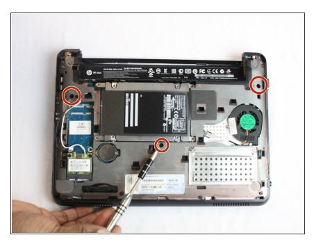
Remove the three black screws marked by the keyboard symbol using a Phillips #1 screwdriver.
