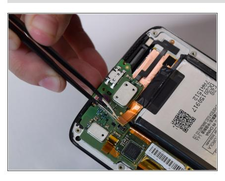
Use the angled tweezers to lift up the small orange plastic piece near the bottom right corner of the battery.
