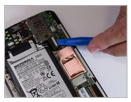
Using a plastic opening tool, unclip the small black ribbon near the upper right corner of the battery.
