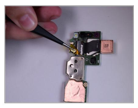
Using the pointed tweezers, remove the tape that covers the ZIF connector.
