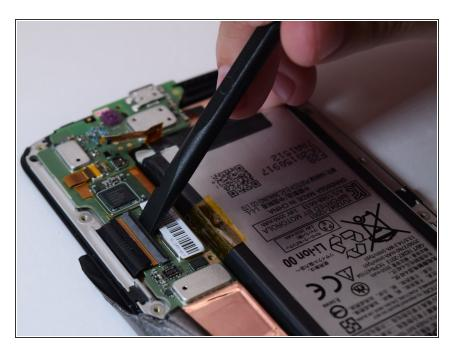
Slightly unlatch the ZIF connector with the spudger. It will pop up, but it will not completely detach.
