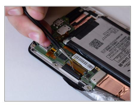
Use the pointed tweezers to remove the transparent gold tape on top of the ZIF connector.
