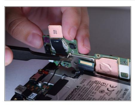
Gently lift up the motherboard and use the blunt tweezers to detach the black antenna cable connector near the top of the battery.
