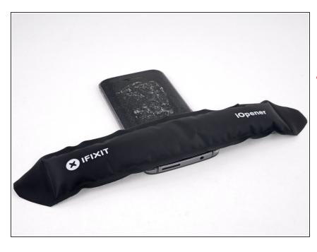
Heat an iOpener and apply it to the top edge of the phone for a minute.
