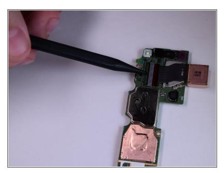
Using the spudger, pry up the ZIF connector.
