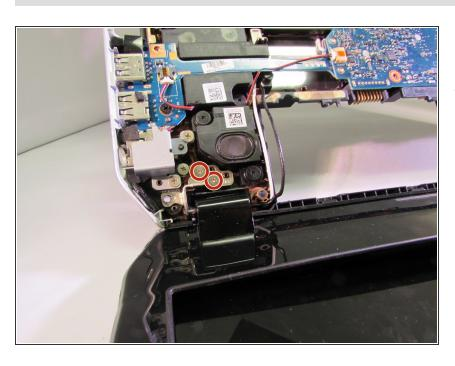
Using a Phillps #1, remove the two 5.6mm silver screws from the base of the first hinge.
