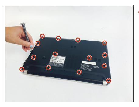
Remove the fourteen 3.75mm screws with a Phillips #0 Screwdriver as shown.
