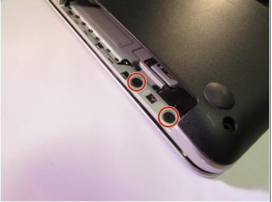
Using a Phillips #1, remove the two 2.4mm screws.
