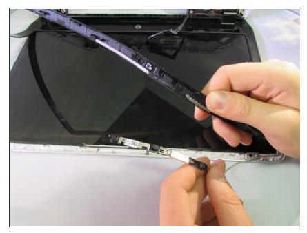
• When prying the screen frame off be careful around the top edge as your webcam will be there. It is a safe idea to move it out of the way like am I doing now.
