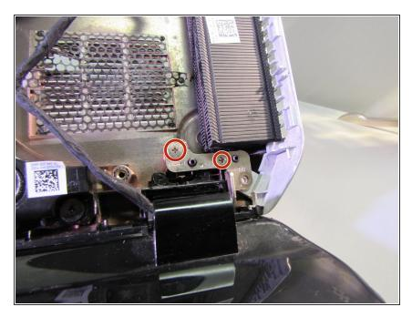
Also using a Phillips #1, remove the two 5.6mm silver screws from the base of the second hinge.
