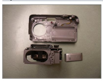
Your battery compartment cover should now be completely removed and ready for repair or replacement.
