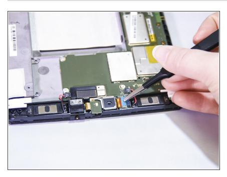
Gently remove the blue tape near the camera using the tweezers.
