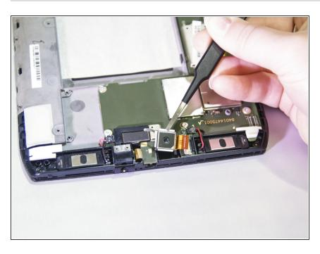
Using the tweezers, remove the camera by grabbing the metal and pulling it out.
