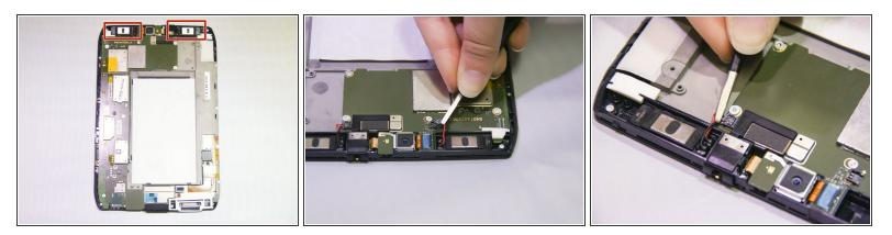
• Using the tweezers, gently pull up the connector of each of the speakers.
