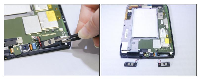
Once the connector is removed, use the tweezers to pull up the speaker from its plastic socket on both of the speakers.
